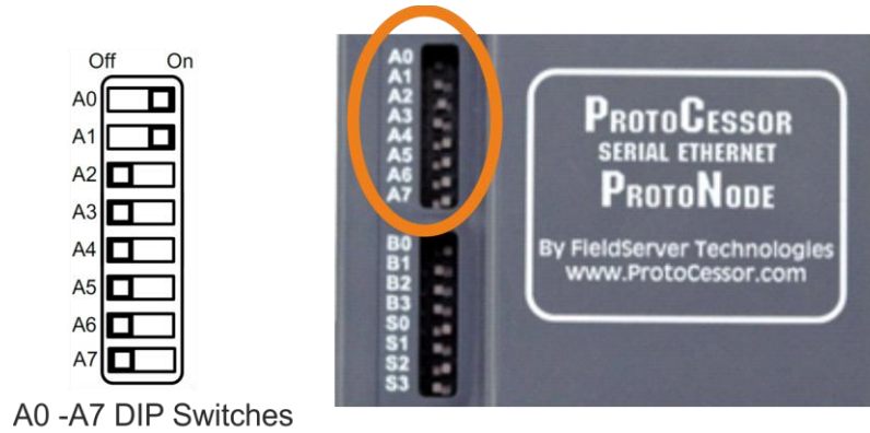
Fig 8: A DIP switches
